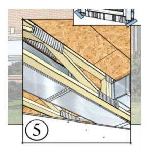
Layout and install all HVAC ductwork to run inside conditioned space to reduce heat loss and improve efficiency.
