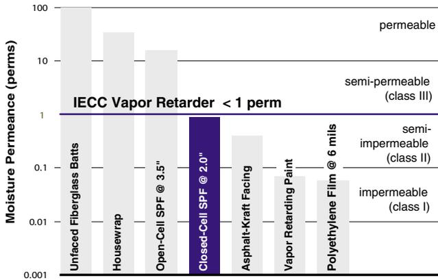
density (0.5 to 0.7 pcf - 8 kg/m<sup>3</sup> to 12 kg/m<sup>3</sup>) open-cell foams have approximately 60 percent open-cell content and offer R-values only between 3.0 and 3.6 per inch at a mean temperature of 75 degrees (ASTM C-518-04). However the open-cell materials are also susceptible to the absorption of both bulk water and moisture vapor. In fact, open-cell foams can absorb in excess of 30 percent water, by volume, which can create an environment for mold and odors.
