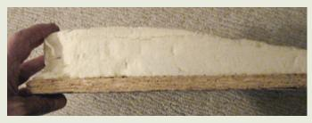
▲ Excessive moisture in the substrate can act as a blowing agent. Here, 2-pound SPF was sprayed on sheathing that was wet on the left side and dry on the right side. The foam on the wet side has increased in volume, compromising cell structure and substrate adhesion.
