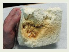
▲ Excessive exothermic heat can actually scorch foam, as shown here, and in extreme cases cause it to catch on fire.
