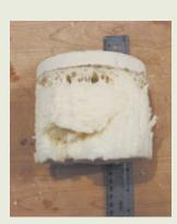
The large void and delaminated area on this core sample indicate that the low-density foam was sprayed on a substrate that was too cold.
