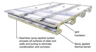
"Environmental control within a building envelope depends on strong interactions between heat, air barrier and moisture transport. ...SPF is an effective air barrier and weather barrier because of its ability to seamlessly fill irregular spaces and provide water resistance."
